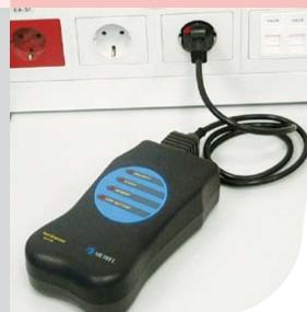
VoltScanner is a 1-phase voltage recorder for testing supply voltage on a socket in accordance with EN 50160 power quality standard.
